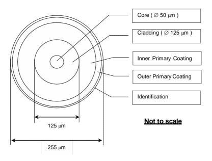
Fig. 1 Cross Section View of Multimode Fiber (50/125, Graded-index)
